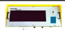
The instrument is Microcontroller based, SWITCH MODE POWER SUPPLY UNIT (SMPS), KEYPAD for programming & Counter setting & resetting, LED display unit for displaying running COUNT. Use of HIGHLY DURABLE SENSING HEAD instead of conventional optical sensors & proximity switches gives better results, longer.
